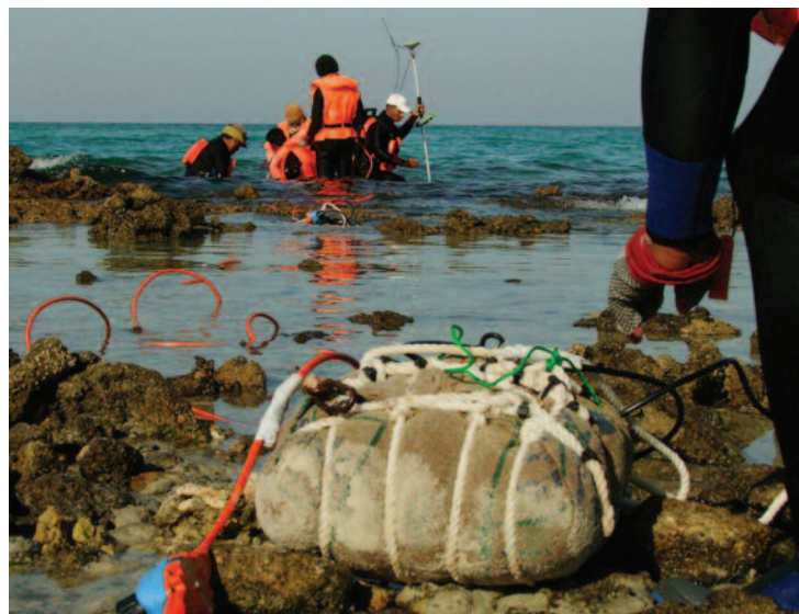
A crew lays out receivers for transition zone operations offshore Qatar. (Photos courtesy of Jaguar Exploration Inc.)
